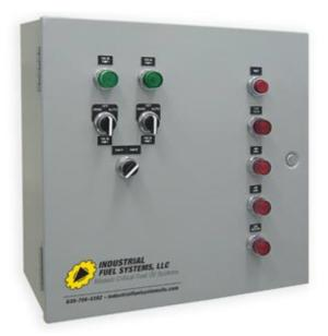
Typical front panel with alarm lights, "Hand-off-auto" switches for two pumps and a lead pump selector switch.
